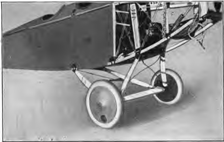
Fig. 100. Landing Gear Installed on Fuselage of Training Biplane.
